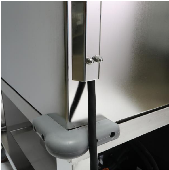
Figure 5. FFU Power Cable emerges on rear of cabinet
