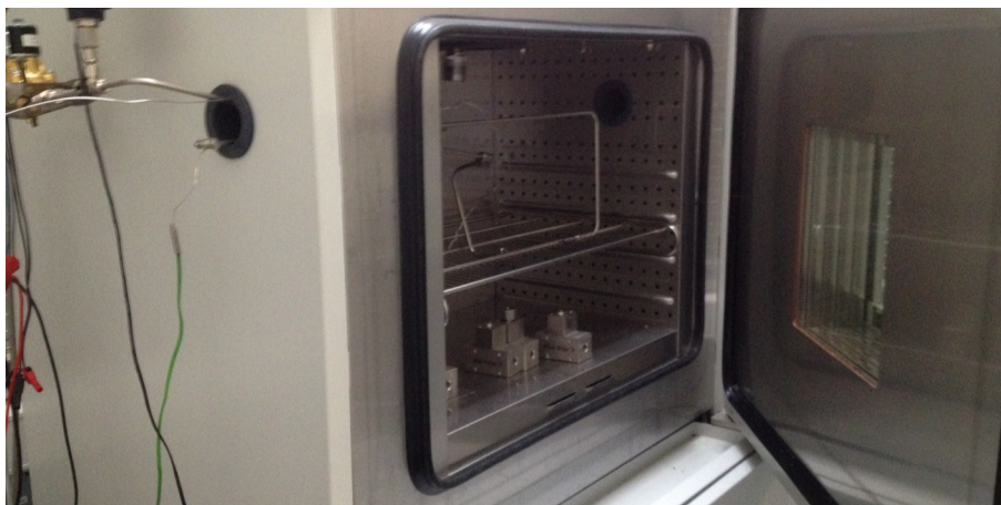
▲ Leaktightness testing of connecting lines under extreme pressure conditions
