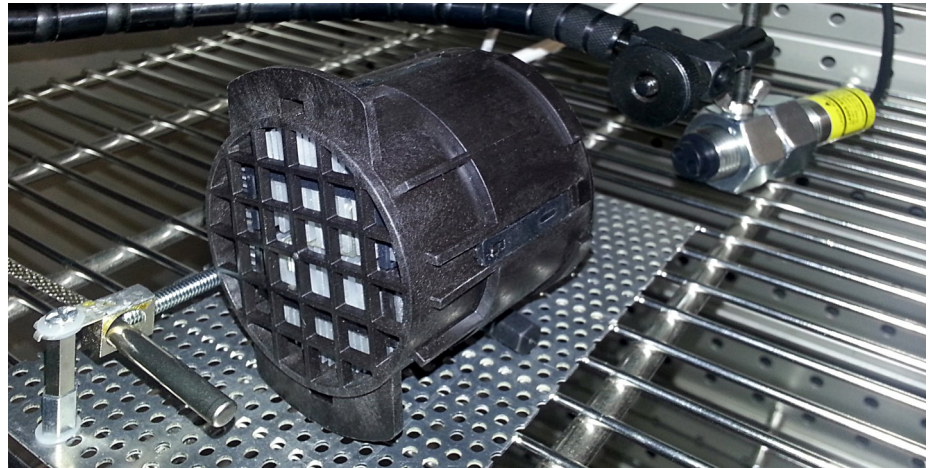
▲ Fan unit with integrated PTC module: Analysis of environmental influences on performance
