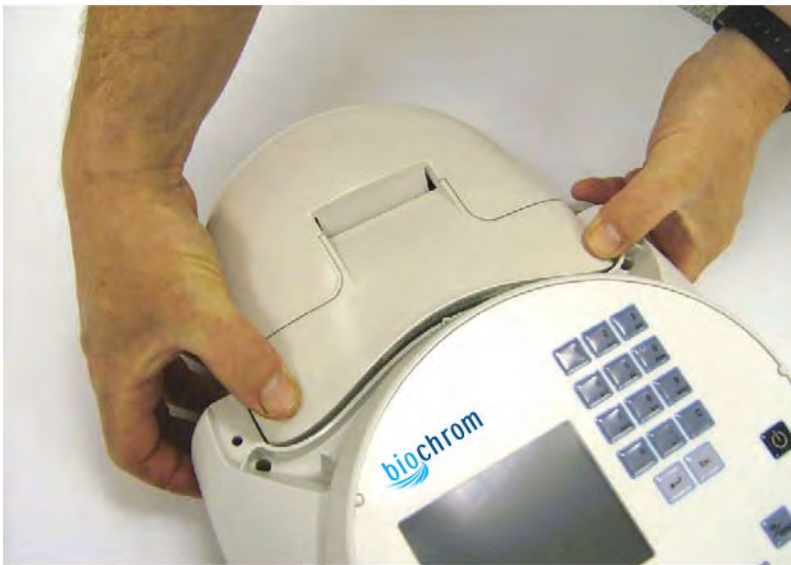
Figure: 16 Step 5. Replace the top cover plate, invert the instrument and replace the cap head screws.
