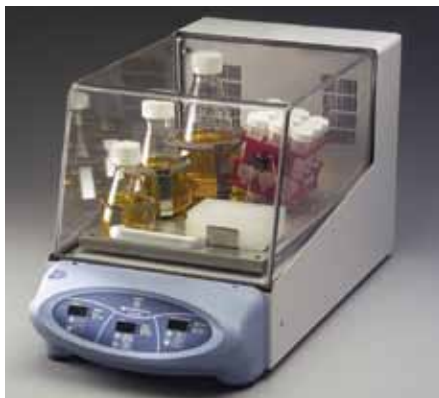
MaxQ 4450 Orbital Shaker by Thermo Scientific Combines incubated/refrigerated temperatures
