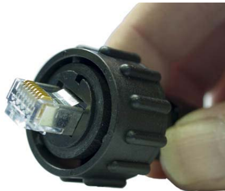
Figure 3-12 Cable Connector Completed
