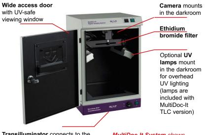
**Transilluminator** connects to the darkroom; UV shuts off when door is open (select from several models)
