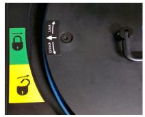
The figure above shows labels that indicate if the sample plate cover is in the locked or unlocked position. Here, it is shown in the locked position.
