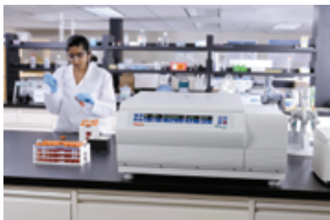
Figure 2 General-purpose benchtop centrifuges offer versatility and convenience, and can be equipped many ways to support tissue culture, DNA/RNA research, cell harvesting, subcellular separations, and many other applications.
