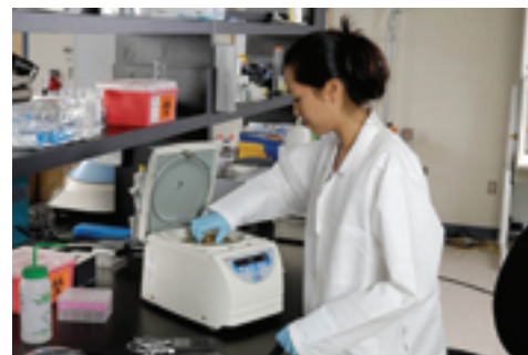
Figure 3 Microcentrifuges are a necessity in every laboratory for everyday microvolume applications such as plasmid, DNA and RNA work, and miniprep kits.
