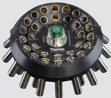
CLINIConic Fixed Angle Rotor, 37°, R max 140 mm
