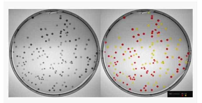
Figure 1: Multi-colony classification using VisionWorks software. After image capture with VisionWorks, the Colony Count Tool was used in 'Auto' mode and two bacteria classes were defined – red represents Serratia marcescens and yellow represents Sarcina aurantiaca. A brief summary of the colony counts is displayed on the screen and corresponds to each class.
