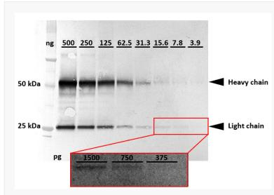
Figure 2: Colorimetric Imaging with the Analytik Jena UVP GelStudio 12 MP Imager. Purified IgG2a was serially diluted down to 3.9 ng for total protein and separated by SDS-PAGE. Proteins were transferred to a PVDF membrane and Western blotting was performed using the Immun-Blot<sup>TM</sup> assay kit from Bio-Rad per the manufacturer's instructions. The inset image contrast and brightness are adjusted to increase resolution of the bands present nearer the limit of detection of the kit.
