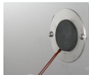
Figure 14: Example of introducing probes through the door space
