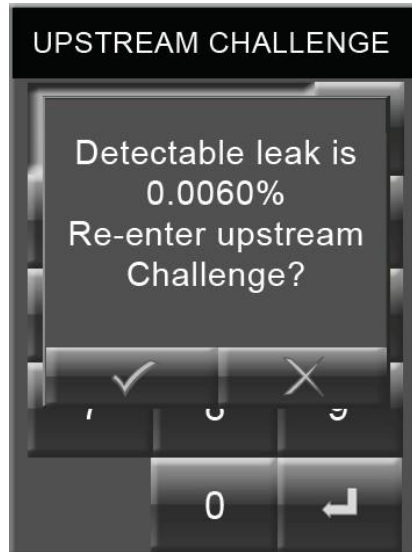
Figure 3-20 Minimum Detectable Leak Screen
