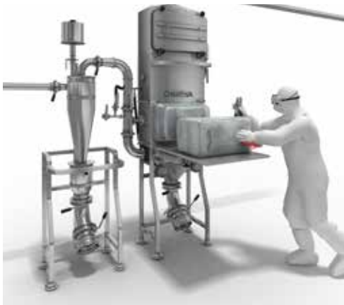
BIBO HEPA REPLACEMENT
