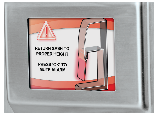
Sash height alarm shown
