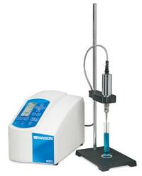
**Stand and Converter Holder:** The support stand with stainless steel rod accommodates Branson's 20 kHz converter. The converter holder supports the ultrasonic stack (converter and horn) and is easily adjusted to properly position the horn in the sample.
