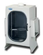
Acoustic Enclosure: Operating a Sonifier<sup>®</sup> SFX Series in the Soundproof Enclosure can minimize mechanical noise produced by ultrasonic processing. The sturdy cabinet is lined with waterproof, sound-absorbing material, which is impervious to most solutions or laboratory reagents and can be easily cleaned. A fully-transparent door enables viewing of the process while limiting the noise to an acceptable level.
