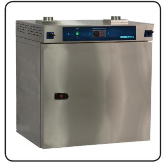
SHEL LAB clean air ovens incorporate all the special features needed for high temperature cleanroom work: a fully welded stainless steel interior, two adjustable perforated stainless steel shelves, rapid heat recovery, and two separate LED digital displays for time and temperature that show setpoint or upto-the-second process information. The Watlow controller is capable of a 40 step ramp and soak profile, or 4 files with 10 steps per file.
