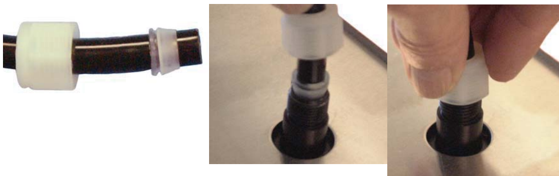
Figure 3-11 Installing Tubing onto Inlet (Example)
