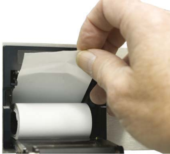
Figure 3-14 Placing Paper into the Printer
