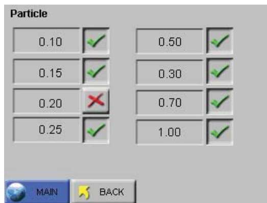
Figure 6-24 Particle Channel Configuration
