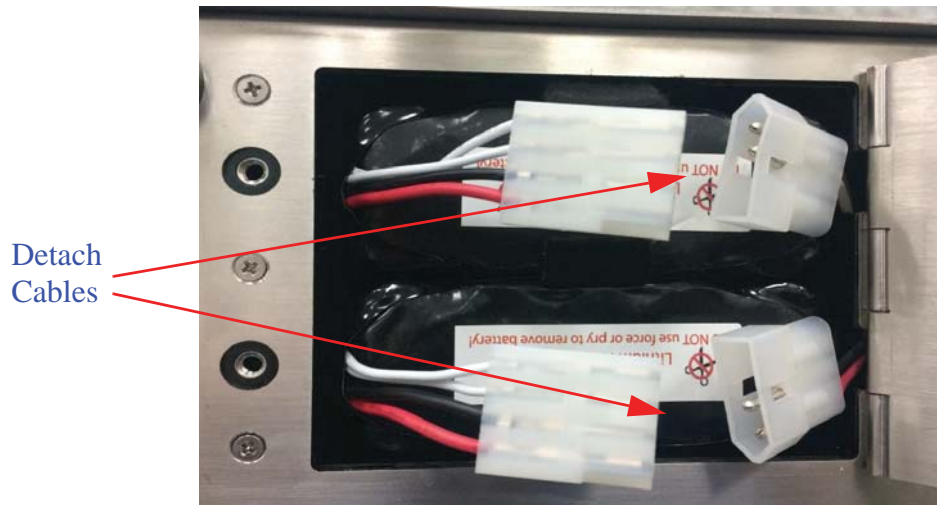
Figure 3-9 Removing Battery (Dual-Battery Units)
