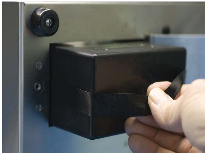
Figure 3-8 Removing Battery (Single-Battery Units)
