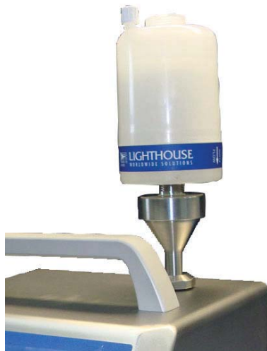
Figure 3-11 ISP Filter Cap Installed
