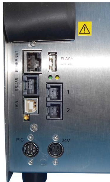
Figure 7-1 The Communications Ports
