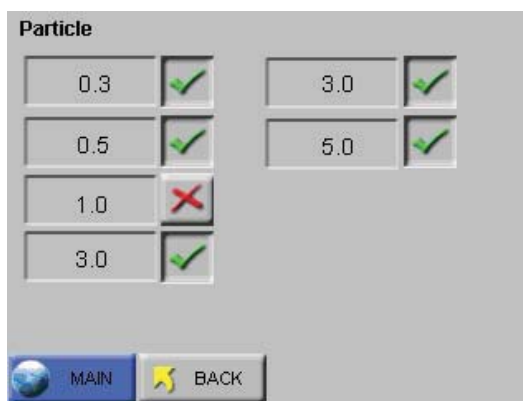
Figure 6-18 Particle Channel Configuration
