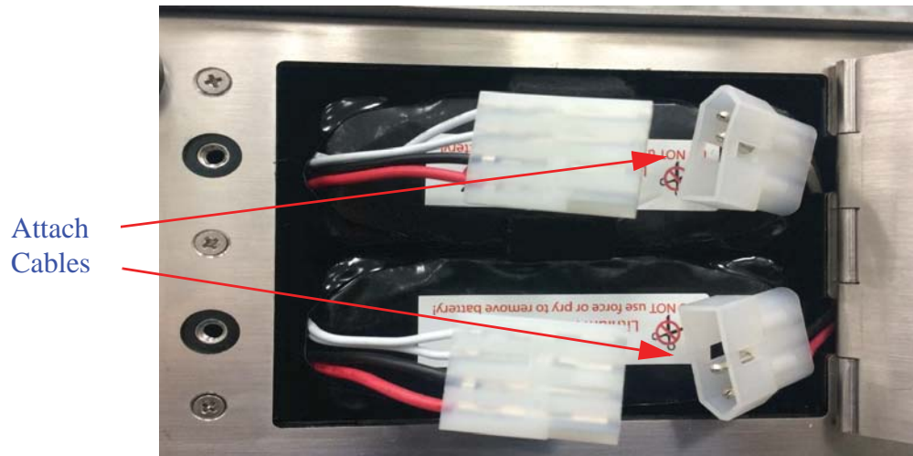
Figure 3-6 Dual-Battery Compartment With Batteries
