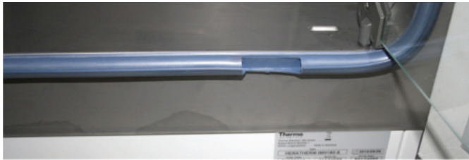
Figure 2: A modified door gasket with a cut out to allow better airflow, thus minimizing condensation in the incubator chamber.
