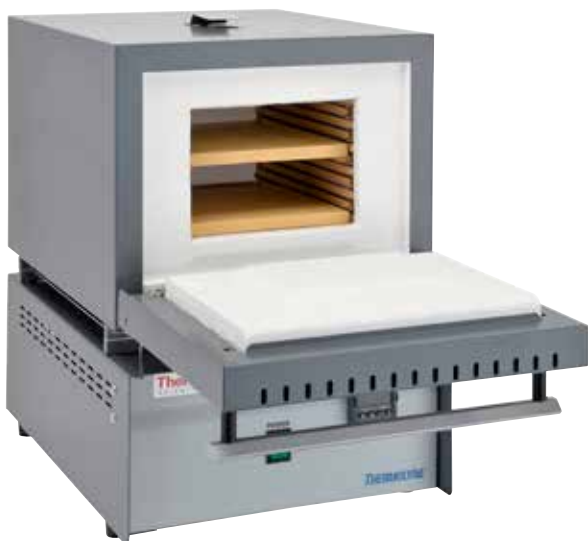
Benchtop muffle 5.8L / 0.2 cu.ft
