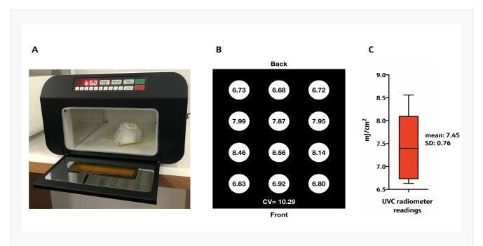
Figure 1. The UVP Crosslinker CL-3000 is a compact, high-intensity, high-uniformity irradiation device. A) Image of the CL-3000 with the front door open and N95 mask placed on the floor of the instrument. B) Diagram depicting the position and intensity of radiometer readings (units mJ/cm²). C) Box whisker summary plot of data from Figure 1B.
