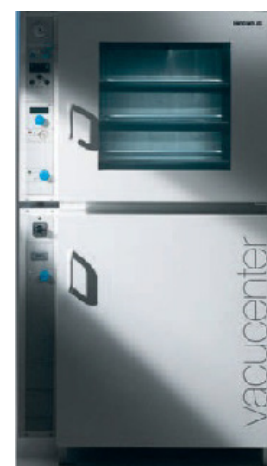
Vacucenter contains pump, oven model VT 6130P on top of unit
